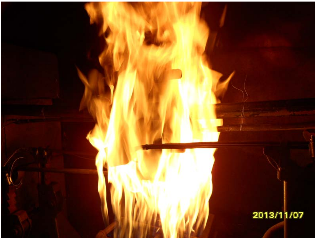
Test Gasket During Burn
