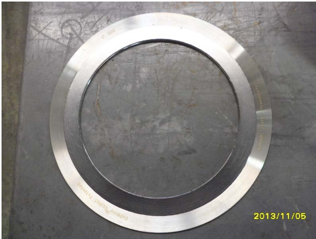
Test Gasket Prior to Burn
